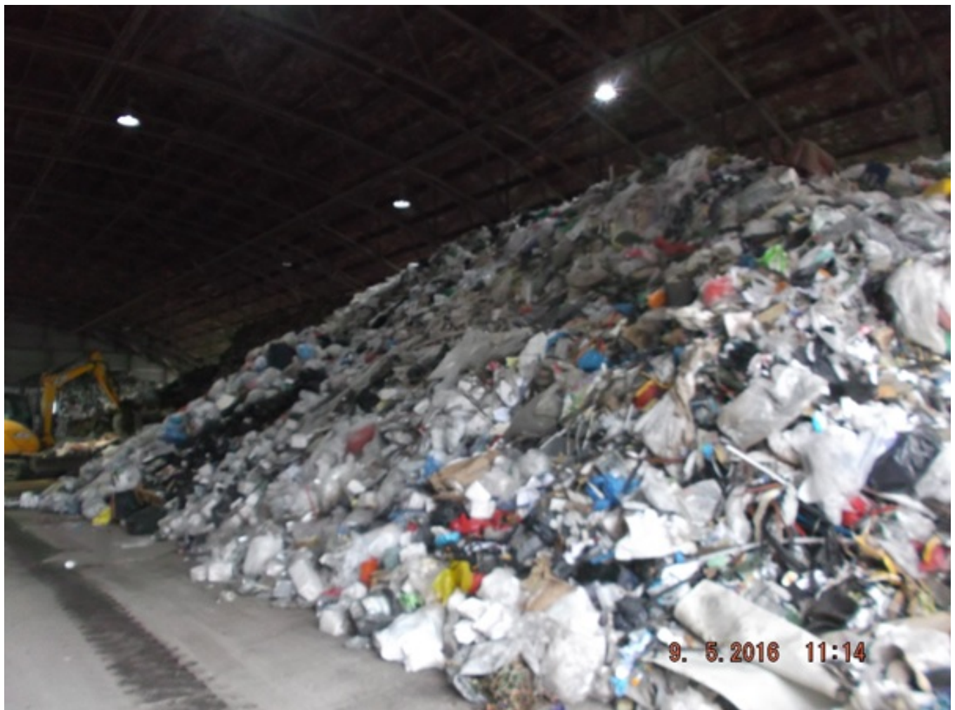
Mixed general waste storage in Hangar B; the pile is joined to another pile of shredded hard plastic
