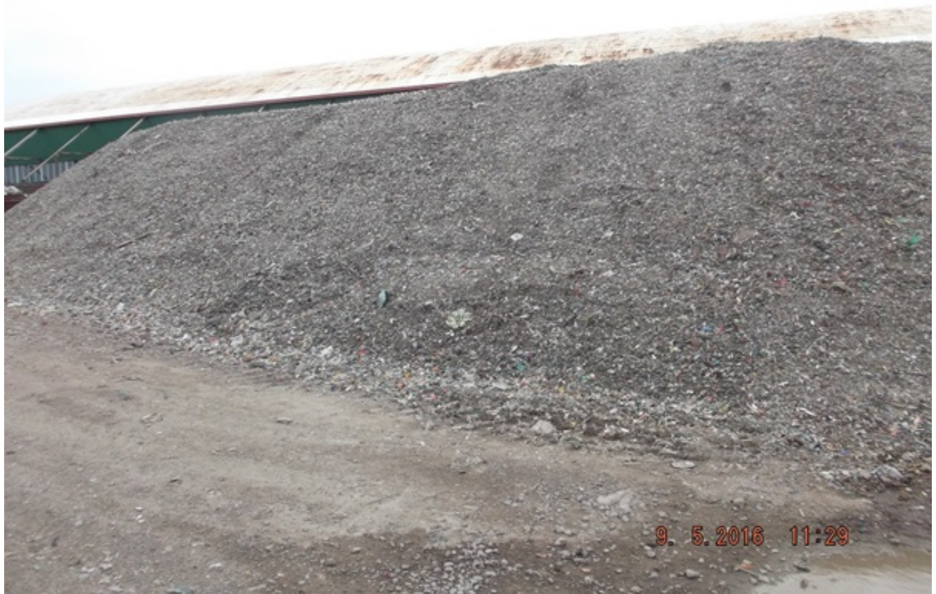
Waste fines stored outside; fines are uncovered, though there is no sign of leachate pooling around material
