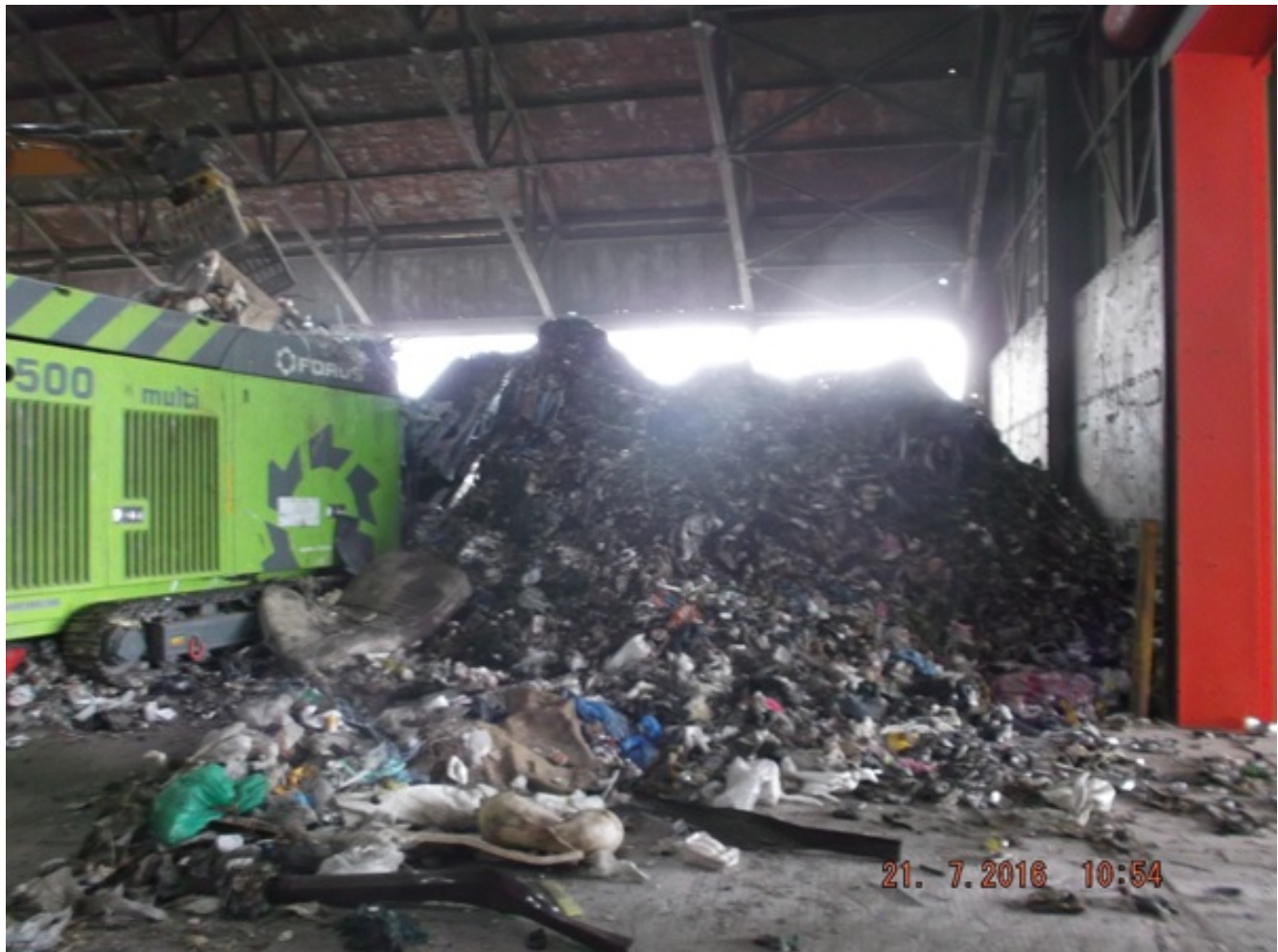
Waste being shredded at the entrance of Hangar B
