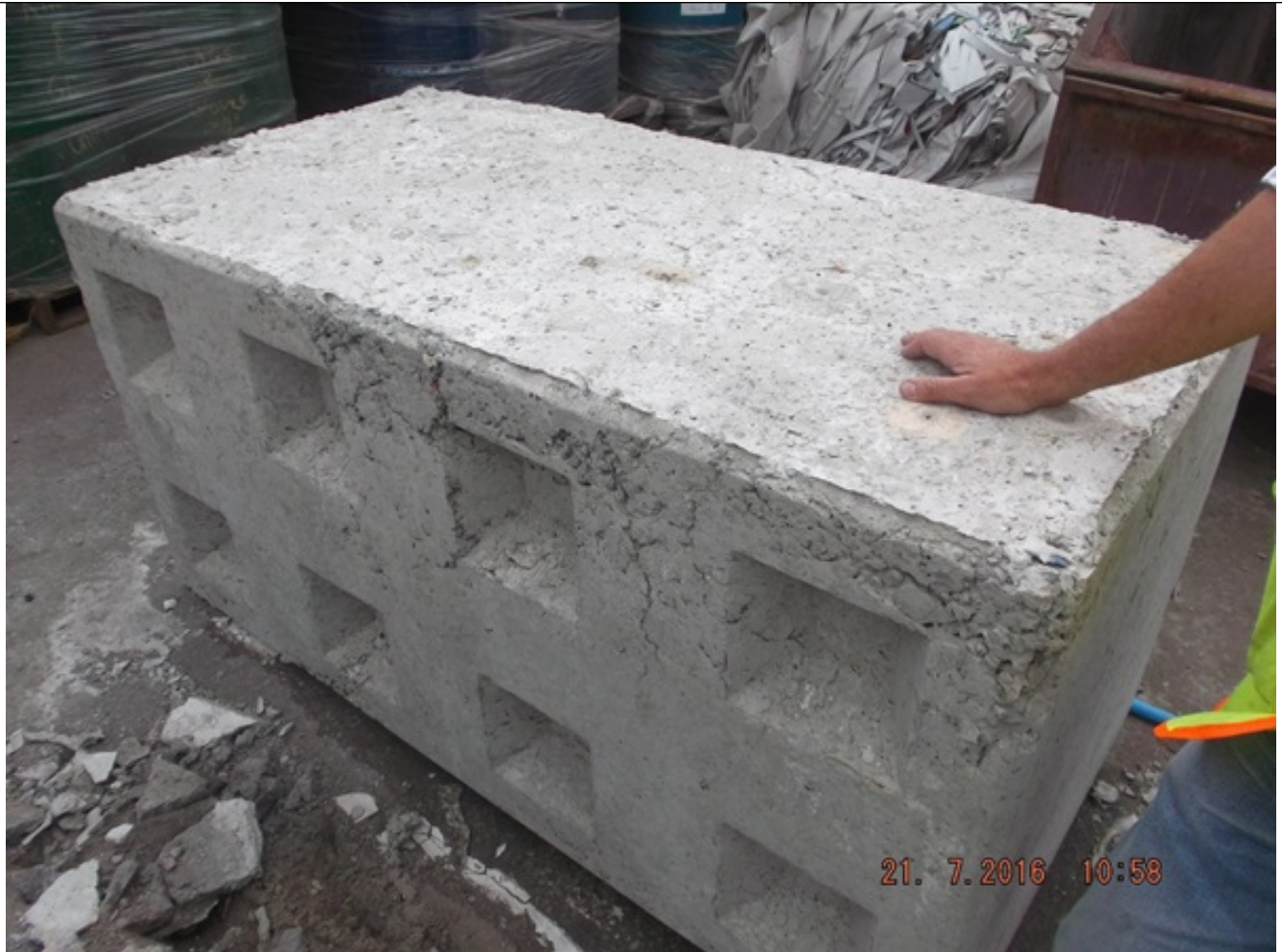
Concrete block produced with 40% mixed waste trommel fines
