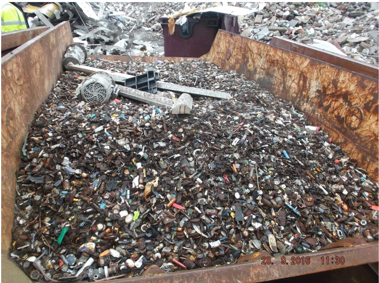
Waste batteries, glass, bottle caps, spent shotgun cartridges and metal fines stored in skips outside. This
