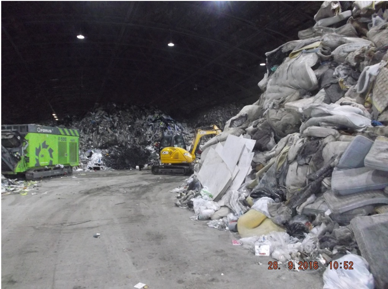
Photograph from the entrance of Hangar B. The pile on the right is mixed waste with a lot of mattresses in. The pile was seen to be steaming underneath the lamps of the hangar.
