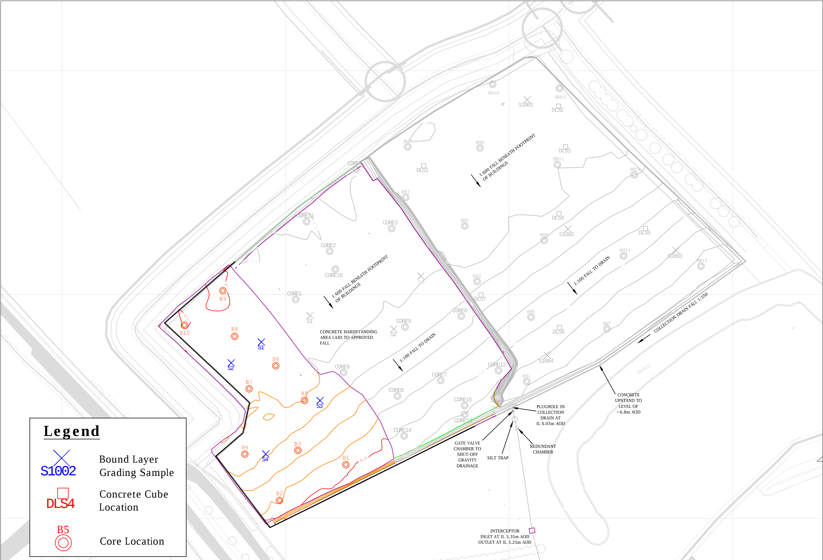
Figure 5 Final Topographic Survey of Slab with Bound Layer Testing Positions
