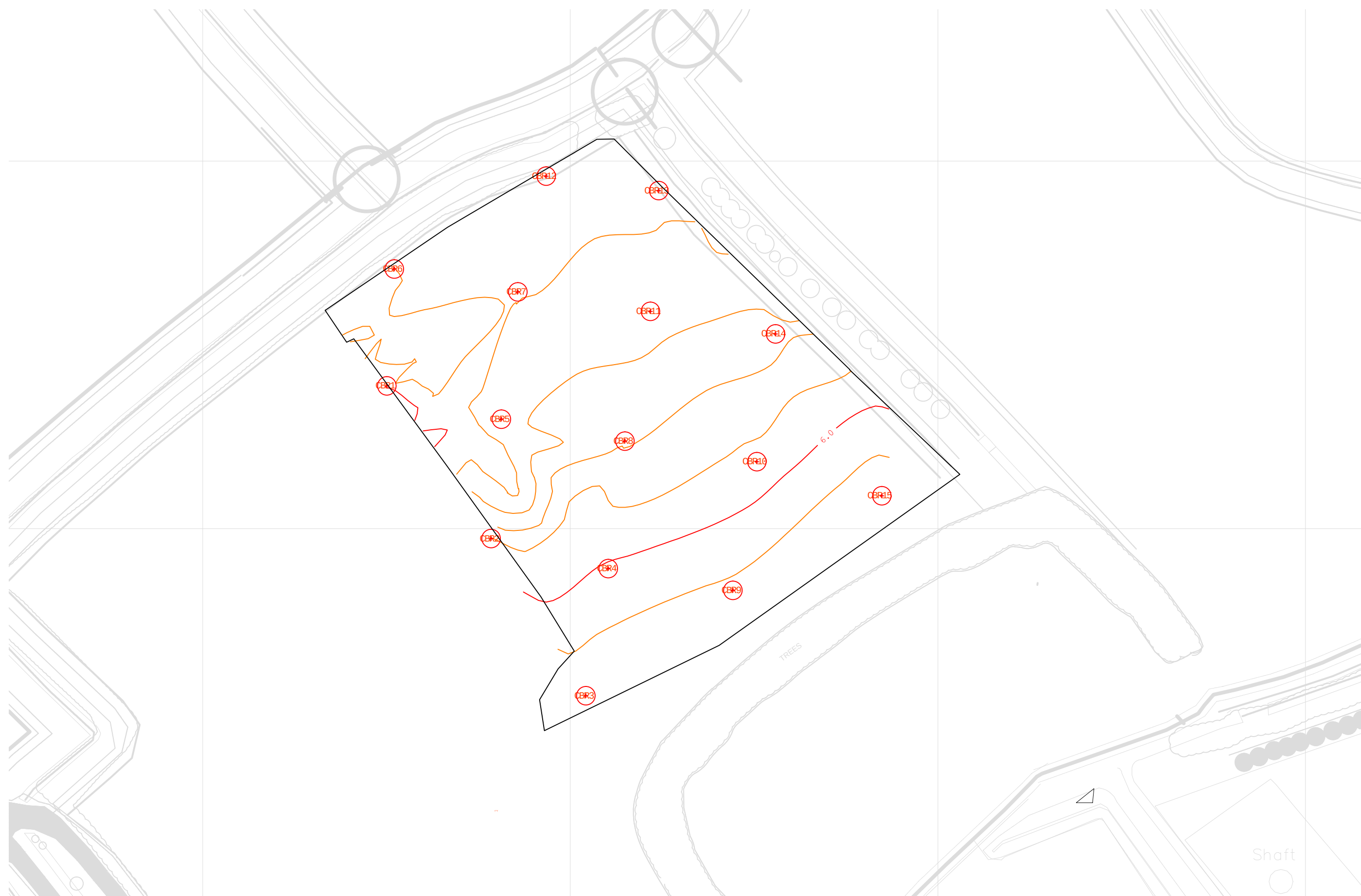
Figure 3 Formation Survey with CBR Testing Positions
