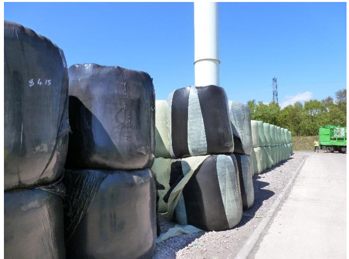
Photograph 3 & 4 – Storage of RDF in tonnages and storage locations contrary to that specified in the environmental permit.
