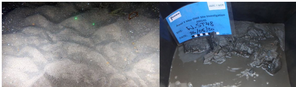
Figure 11: Sediment images from the offshore extent (right; sample W_ST13_03)) and south-east (left; sample W_ST48) of the ECC, as captured during the project specific survey (Fugro, 2020a).
