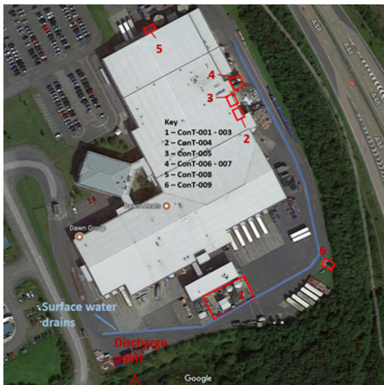
Plate 1 - Location of bunded areas and drainage system
