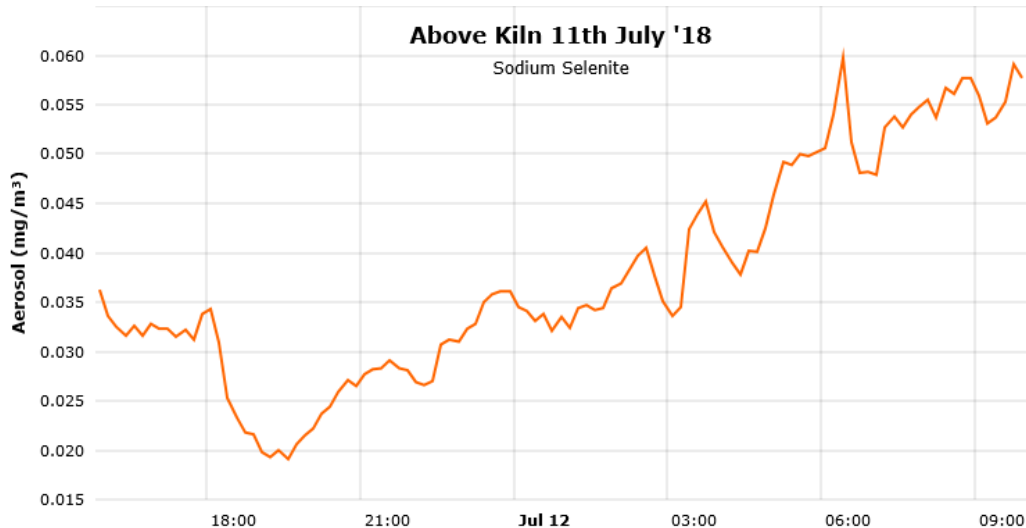
Figure 4: Photometric results of ambient PM concentrations at the front of the Kiln during the production of Selenium Boluses using sodium selenite as the raw material.
