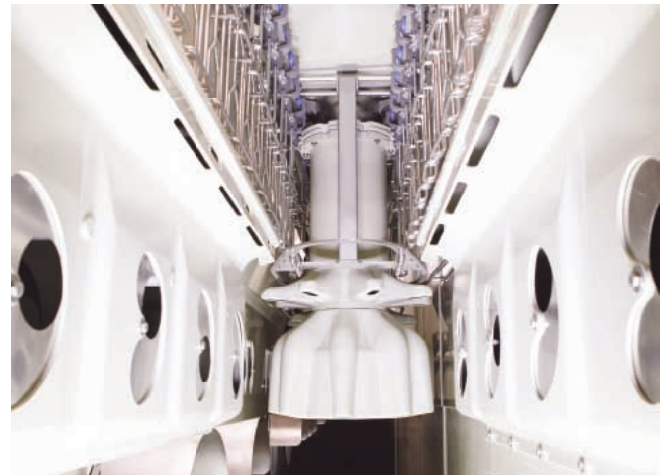
The airflow on the carcass is adjusted for perfect scald results.
