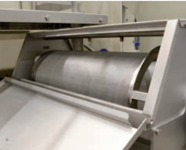
Recycling and filtering un-absorbed water reduces water and energy consumption.
