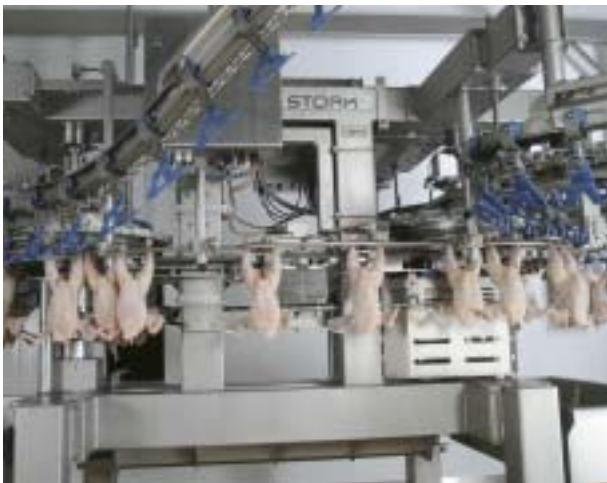
The weighing re-hanger gives the weight of each bird passing into the chilling tunnel.
