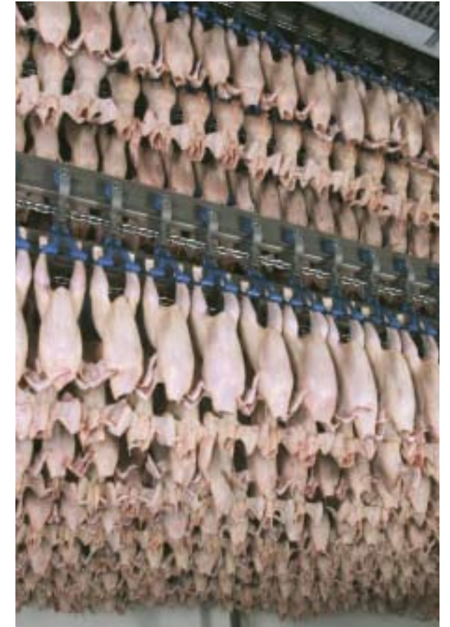
Downflow 'Plus' is a single-stage multi-tier system.
