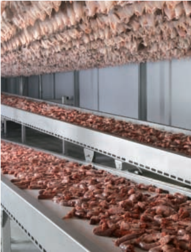
An alternative to chilling giblets in water is a conveyor belt system in the air chilling tunnel.
