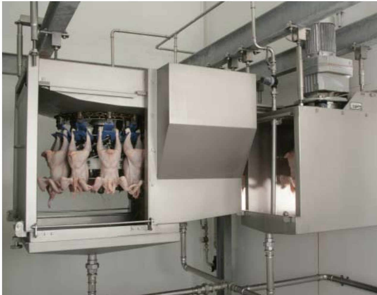
A moistener and spraying cabinet keep yield loss to a minimum.
