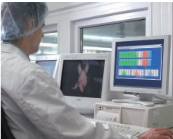
Stork's product distribution system (PDS-NT) tracks all birds, flock numbers and weights through the tunnel.
