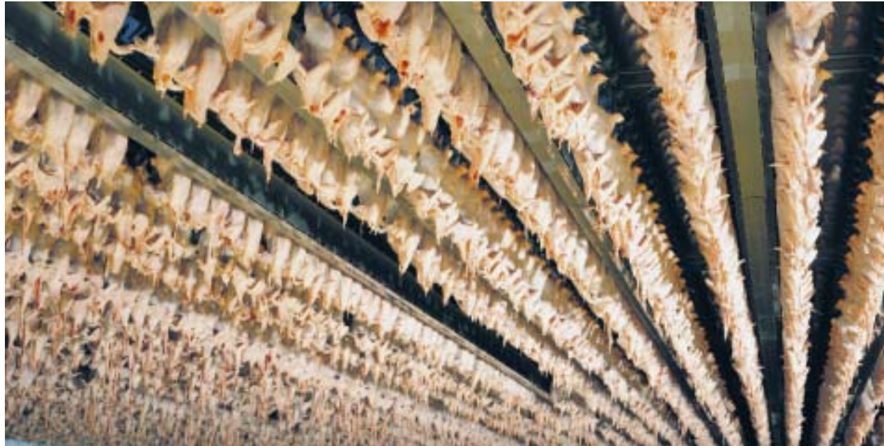
An InfraChill tunnel is a single-stage single-tier system.
