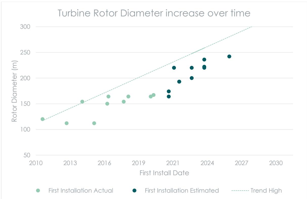
Figure 2 Construction of new, larger, WTG models over time, shown by the date each model was first installed (source: RWE via publicly-available information).
