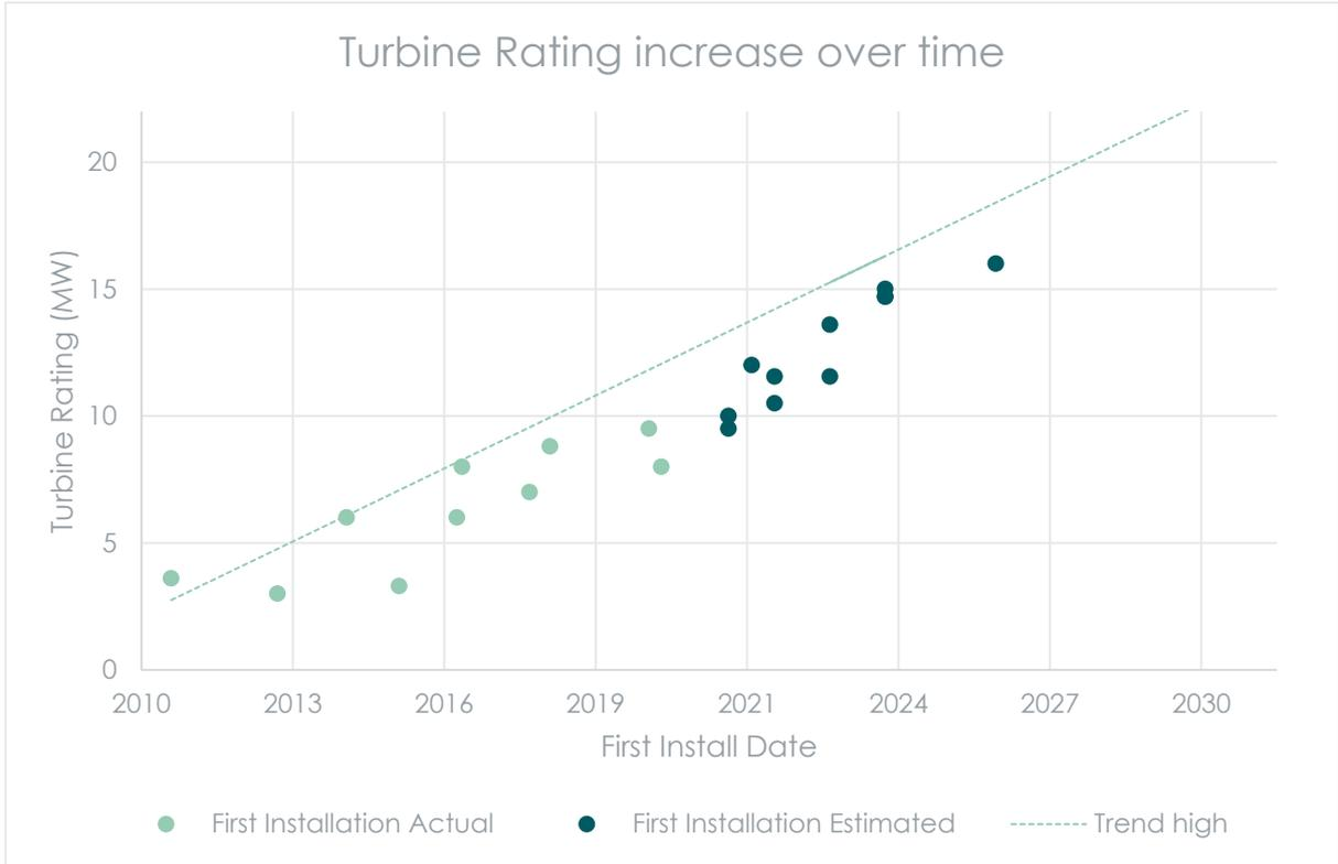
Figure 1 Construction of new WTG models over time, shown by the date each model was, or is planned to be, first installed (source: RWE via publicly-available information).
