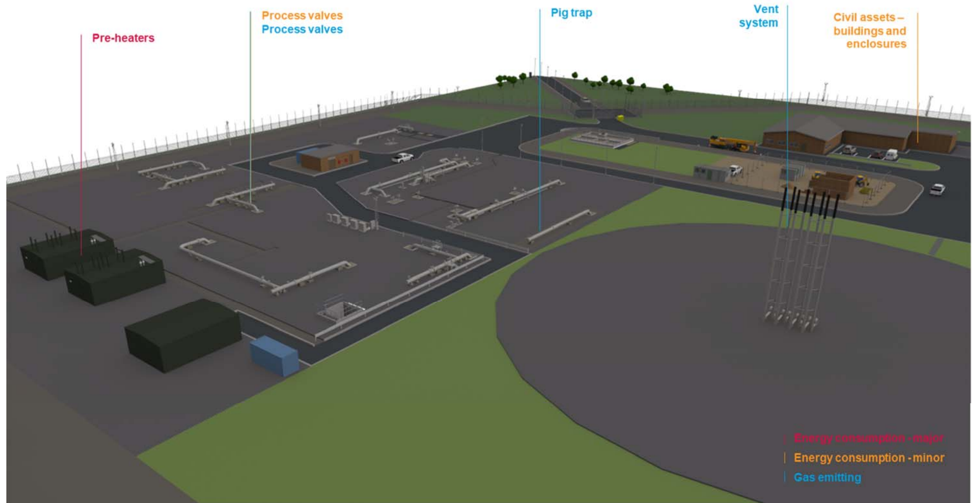
Figure 7 Generic compressor station site illustrating NTS SACs
