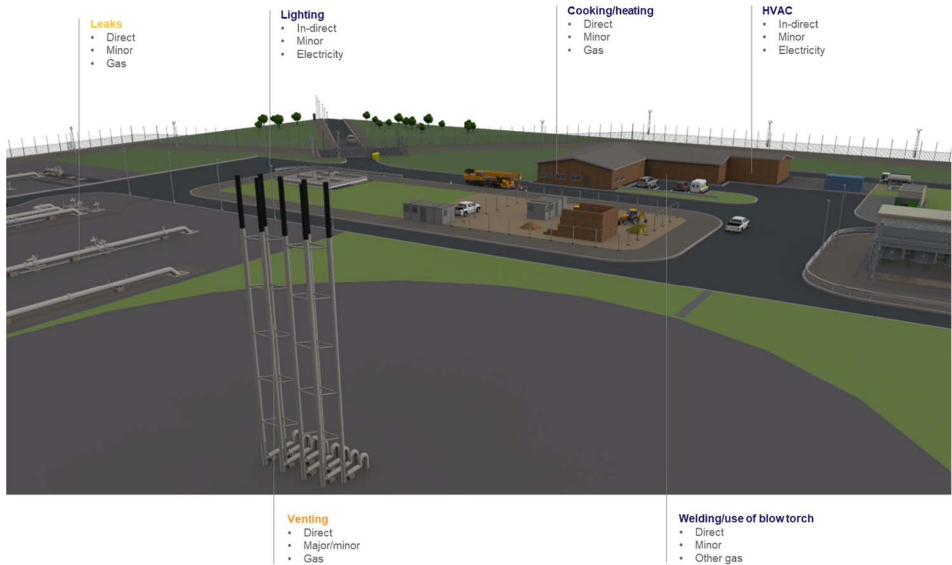
Figure 5 Generic compressor station site illustrating activities and associated energy consumption
