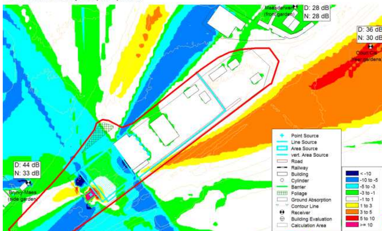
Figure 9: Calculated noise map of predicted level difference ( \Delta L dB) between unmitigated and mitigated Recycling Facility daytime peak noise emissions
