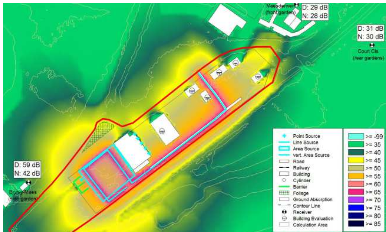
Figure 5: Calculated noise map of predicted early morning recycling facility noise levels ( L_{Aeq,15min} dB) without mitigation
