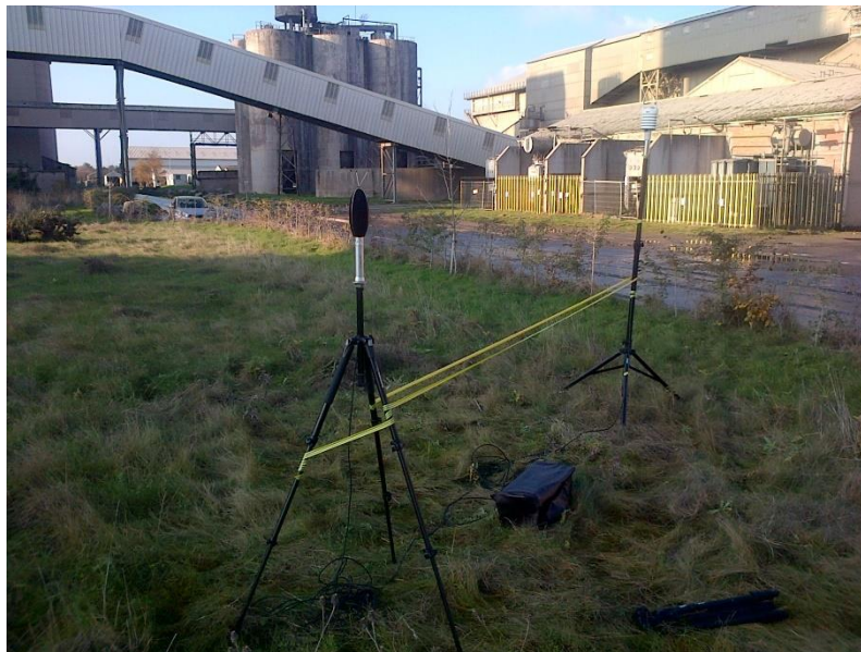
Figure 4 – Photograph of SLM and weather station at Castle Cement
