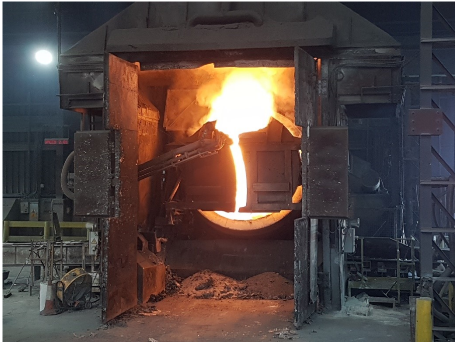
Figure 1: Rotary Kiln Furnaces Showing Hood Extraction
