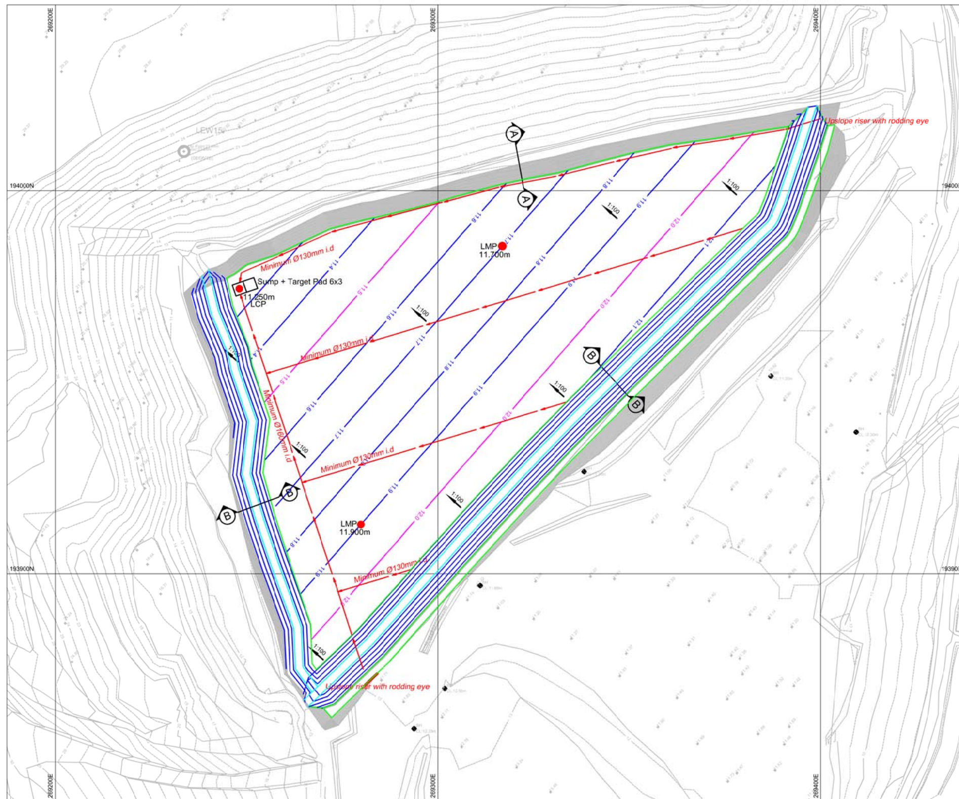
TOP OF CLAY LEVELS & LEACHATE CONTROL SYSTEM
