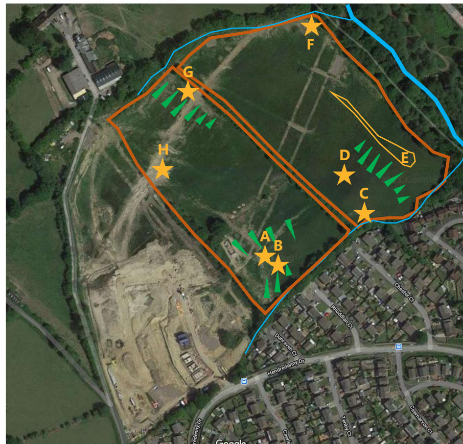
Figure 2-1 Seeps and springs (yellow stars) and slope features (green triangles) noted during walkover March 2021
