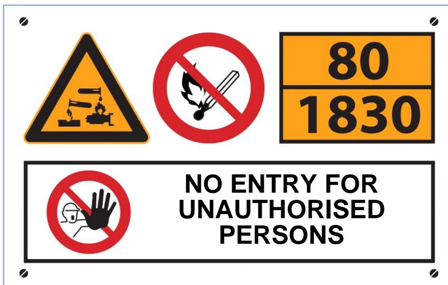
**Figure 6: Safety sign for the sulphuric acid space**
