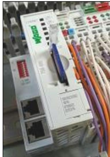
Figure 51: Wlogger with SD card
