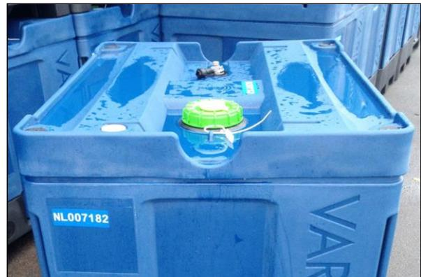
**Figure 12: Double-walled acid tank**
