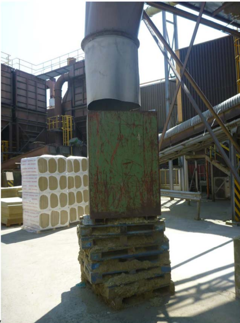
Photograph showing extensive wool waste (from PSM 56 cutting section) covering the external yard. Arrow denotes drain.
