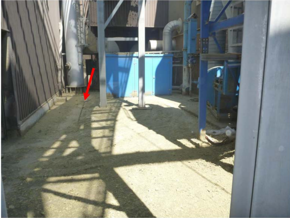
Photograph showing extensive wool waste (from PSM 56 cutting section) covering the external yard. Arrow denotes drain.
