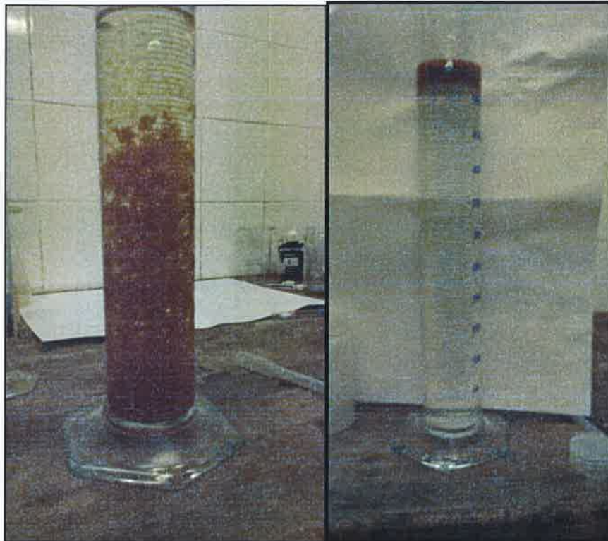
Figure 1: Formation of hydroxide solids through pH adjustment and floating by use of simulated DAF
