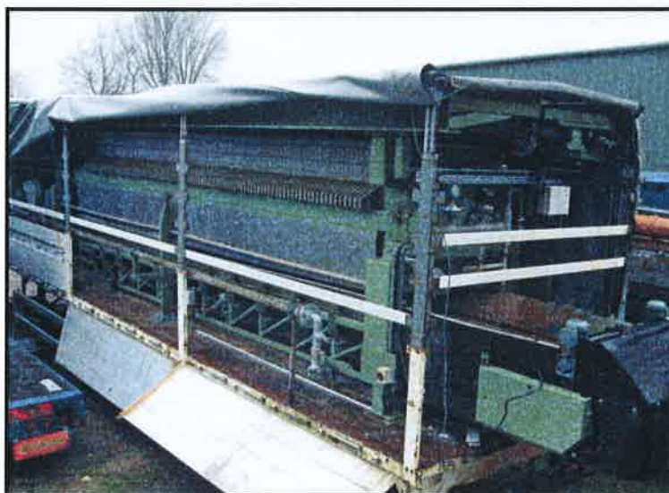
Figure 2: Trailer Mounted 2.8m 3 filter press
