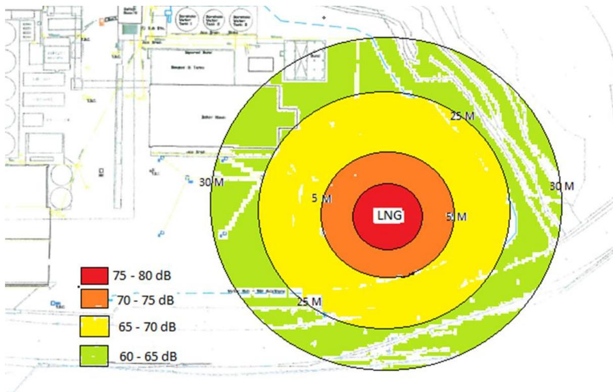
Significantly the noise emitted from the delivery pump was considerably lower than the 85dB listed within the specification document, the noise levels recorded were more like 85dB at 2m from the delivery point.
