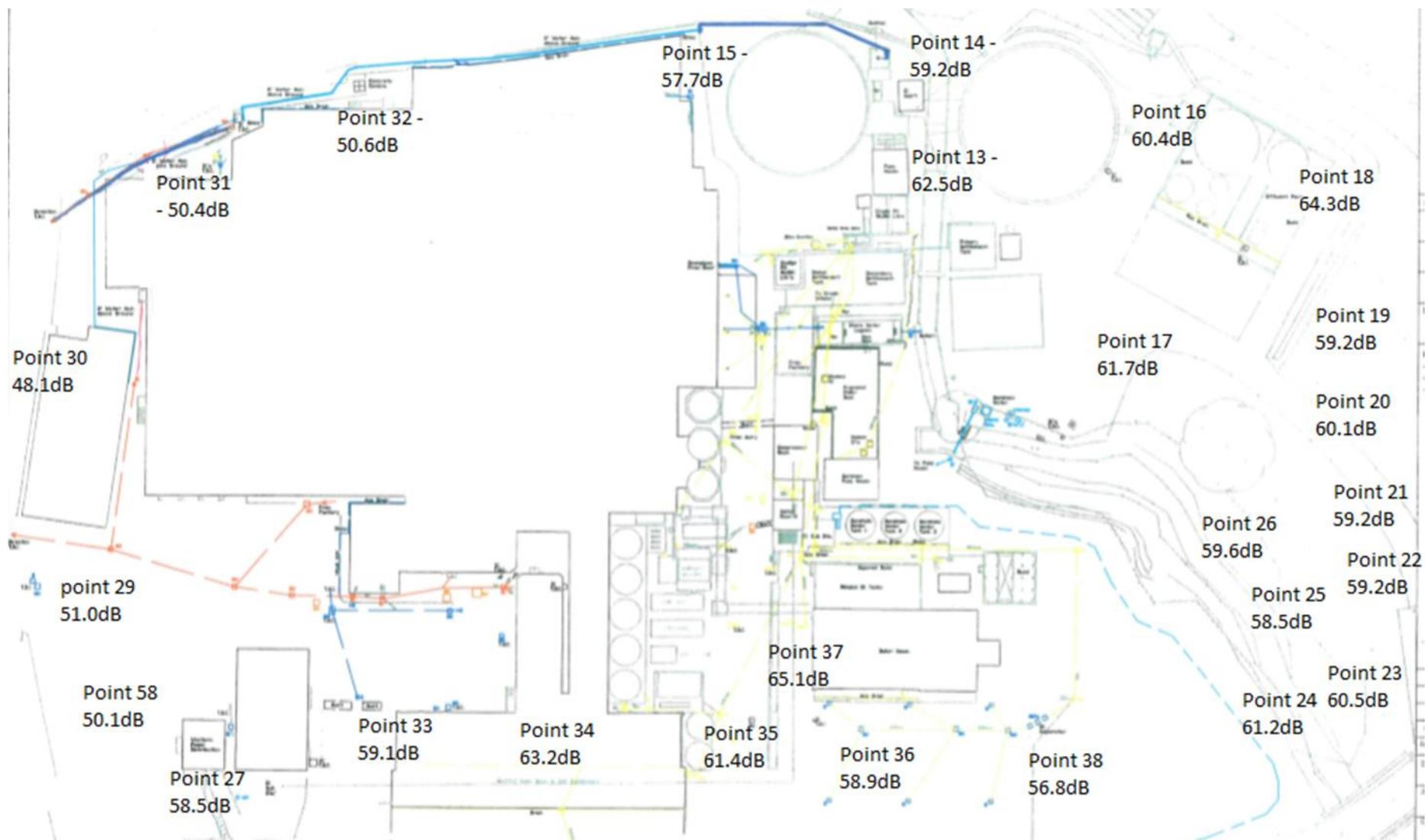
38 sample points, were chosen across the site to cover all aspects of normal operations, each point was monitored for three mins to obtain a time weighted average, at this point no further in depth investigation of the data has taken place, this was a spot check of the operational noise generated during a normal production day.
