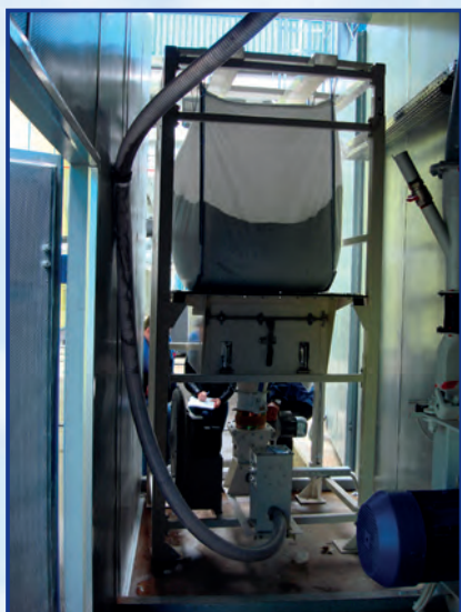
A one-tonne big bag feeder injects absorbent
