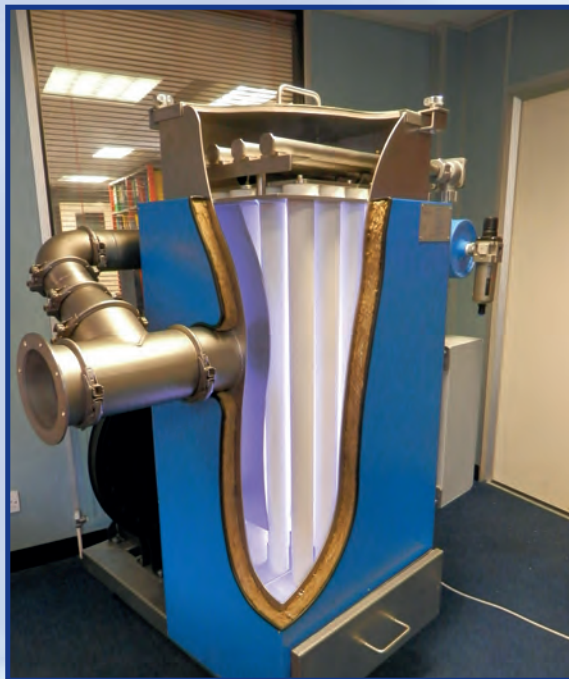
Section of a BMF filter
