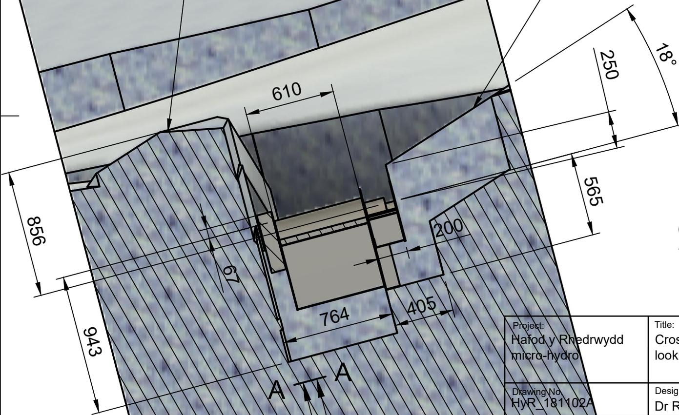
Cross-section at 1:25 scale
