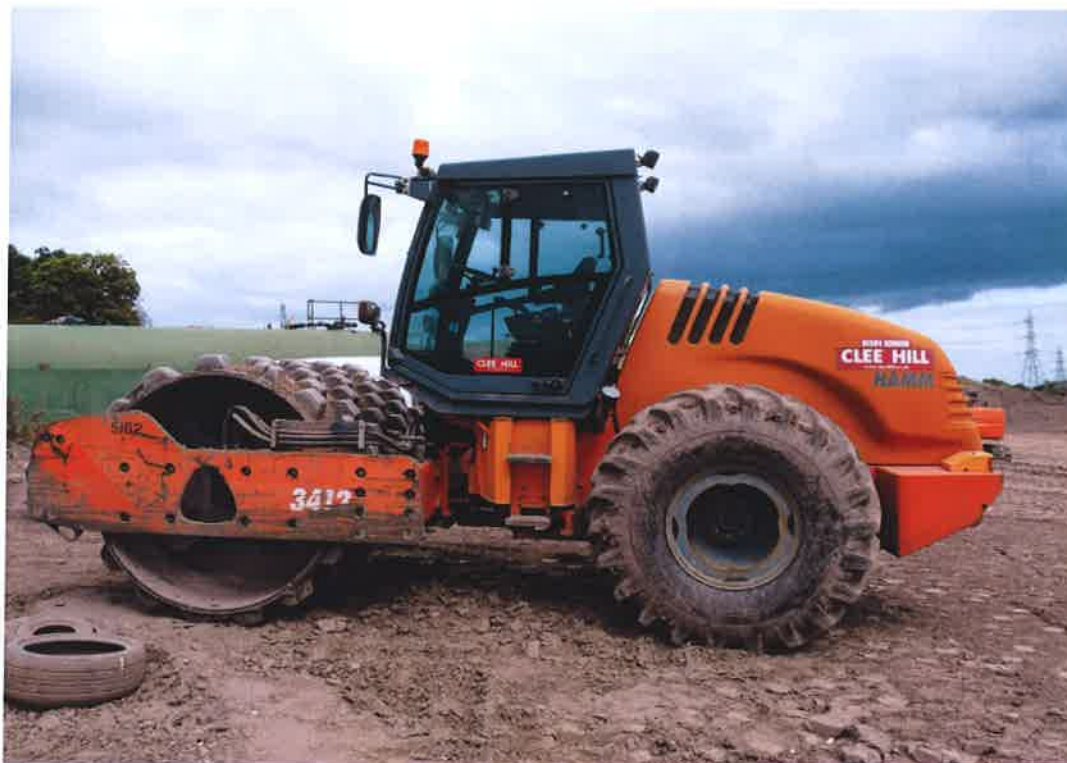
Padfoot roller utilised for cell construction (Hamm 3412)
