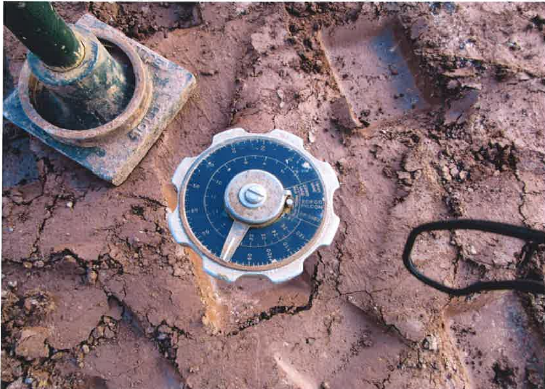
Hand shear vane and undisturbed core samples taken to confirm clay suitability
