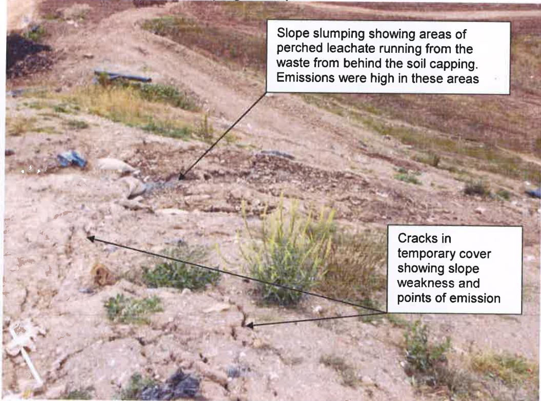
PHOTO 2: Cracking and Slumping of Slope
