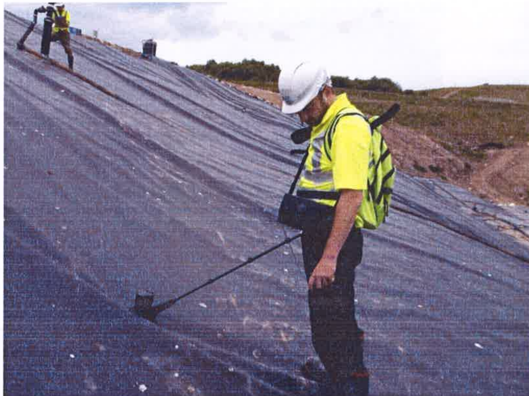
PHOTO 3: Emission From Extrusion Weld in Boot Detail
