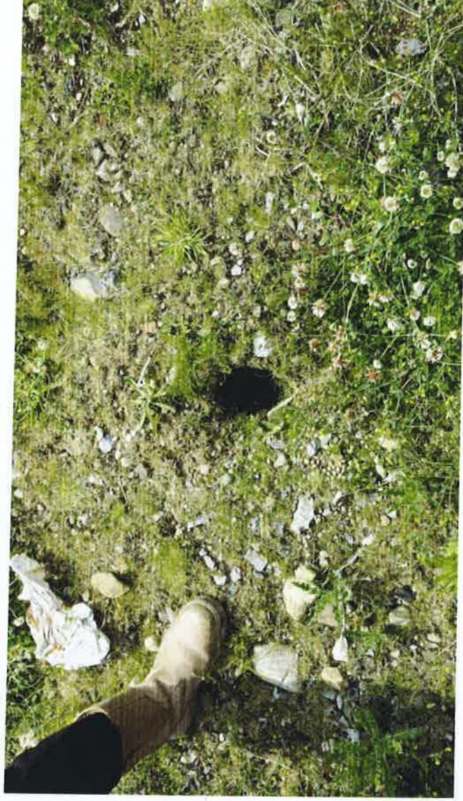
2. Rabbit Hole? High methane emissions (9000ppm). 2011 Capping works
