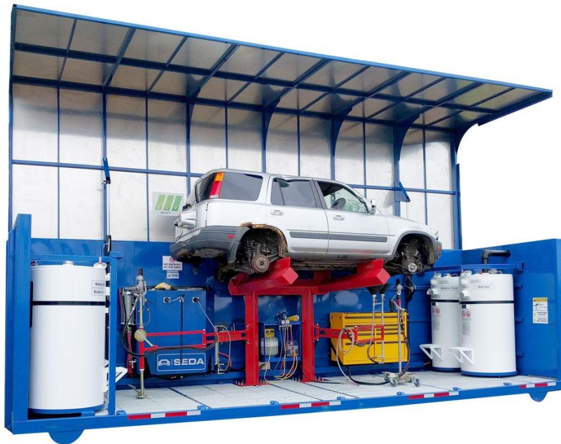
Photograph 5-1: Containerised ELV drainage system
