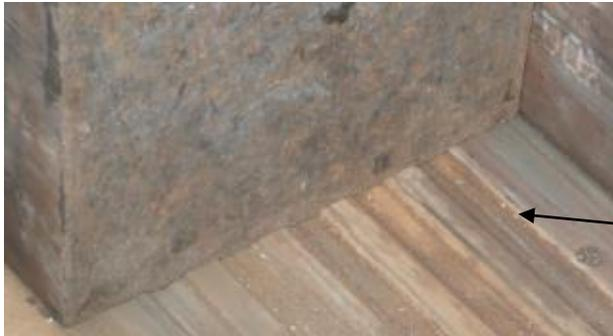
The pusher piston rests on grooved wear plates made of **HARDOX 500**. The rod of the pusher cylinder is thus particularly protected against the risk of scratching related to the return of scrap.
