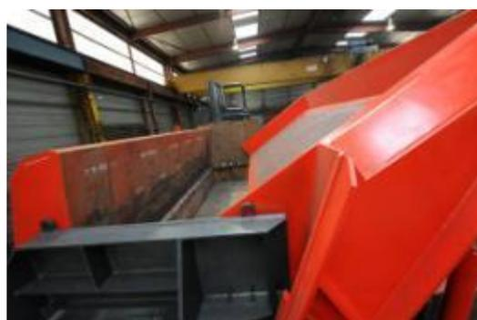
Through its innovative kinematic design **the loading bucket is able to discharge the scrap directly under the lid**. The number of movement of the lid and side-press piston is reduced allowing a fast closing of the box.
