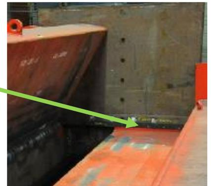
The analogue detection of the side press piston movements is made by means of a laser remote measuring sensor fully protected against any risk of chock during handlings of scrap.
