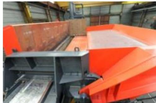
The loading bucket allows to load the scraps as a background task and facilitates a qualitative sorting of the materials.
