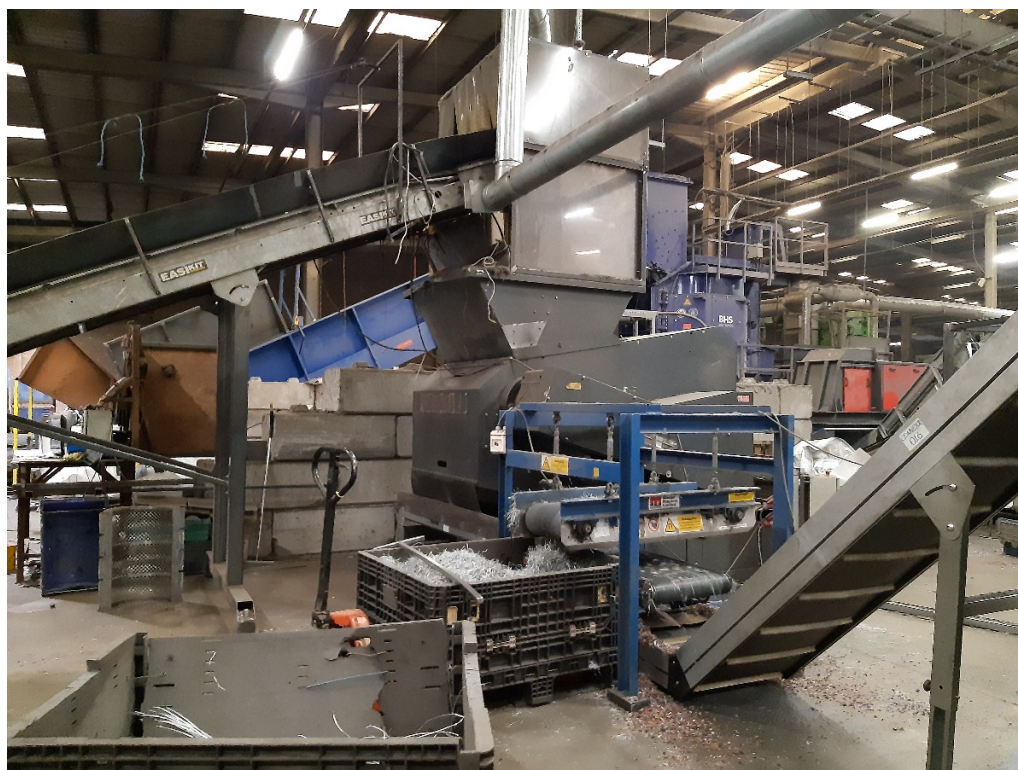
Photo 5 (below) – An electrostatic separator has been installed to separate conductive and non-conductive materials (less than 10mm)
