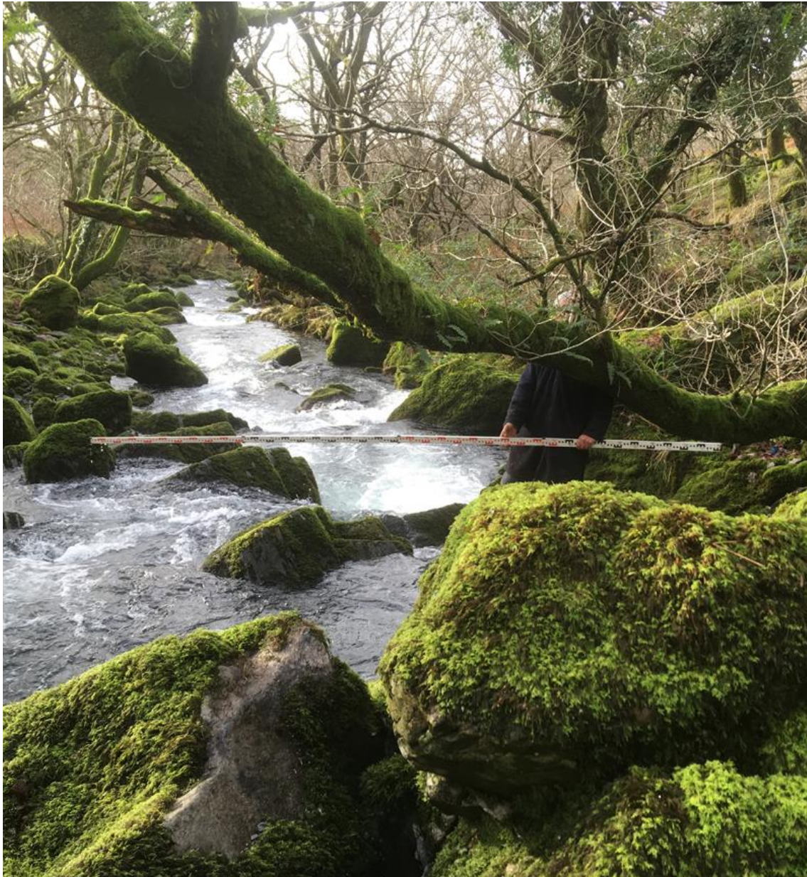
Figure 6. View downstream from proposed intake position. The staff indicates the height of the proposed weir crest level
