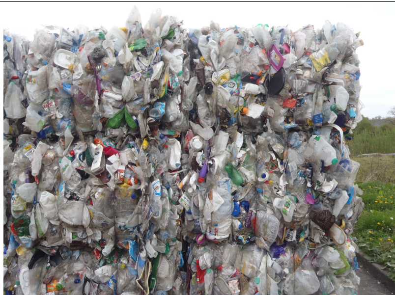
Plastic bale with visually a very small amount of non-target material
