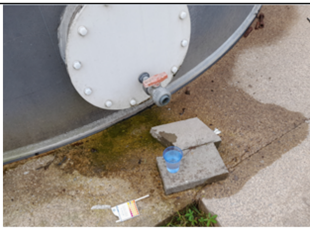
Site testing showed this to be neutral condensate
