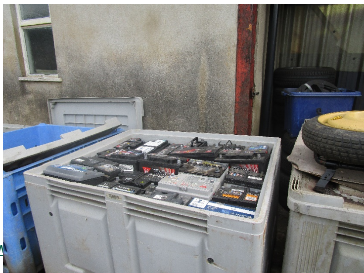
Figure 5. Waste batteries stored in an acid-resistant container (lid placed next to it)
