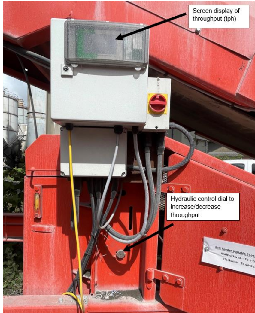
Figure 4: Weigh feeder adjusting point and weight indication screen
