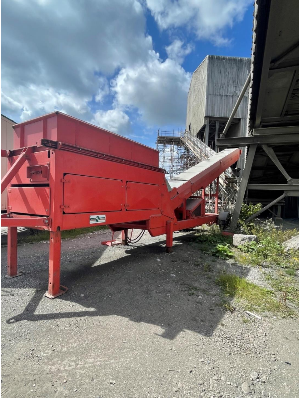
Figure 3: BFS loading hopper and conveying system into cooler building
