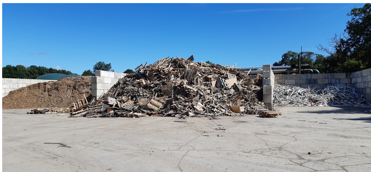
Photo 4 - Stockpiles of wood waste(s) stored within segregated concrete bays
