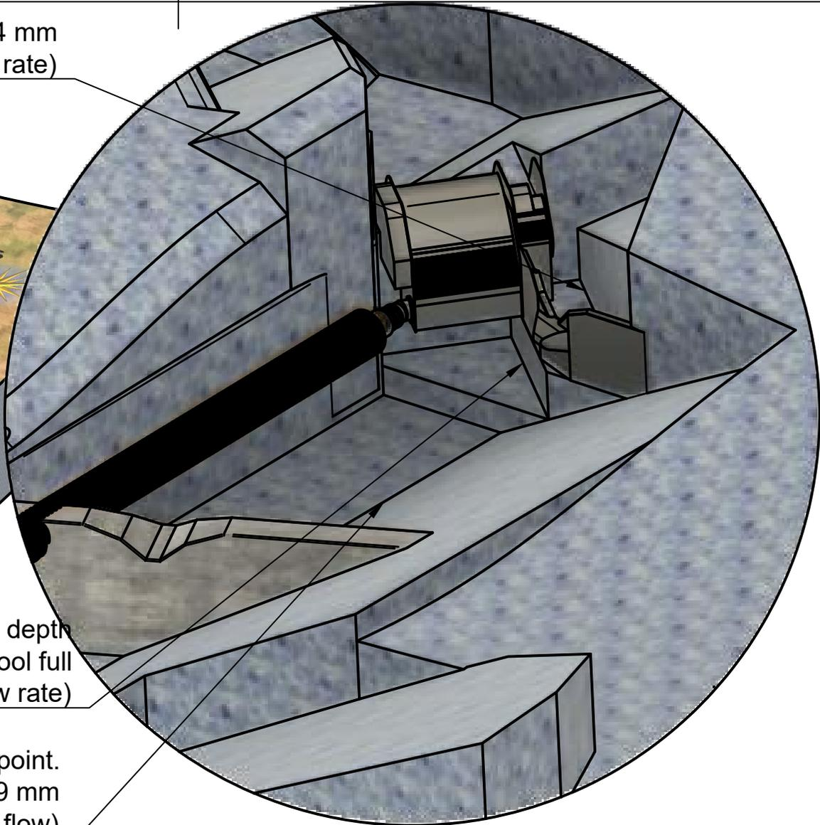
Cut-out datum 420.83 m, minimum water depth below CBS050 screen 358 mm (pool full to barrage notch, zero flow rate)
