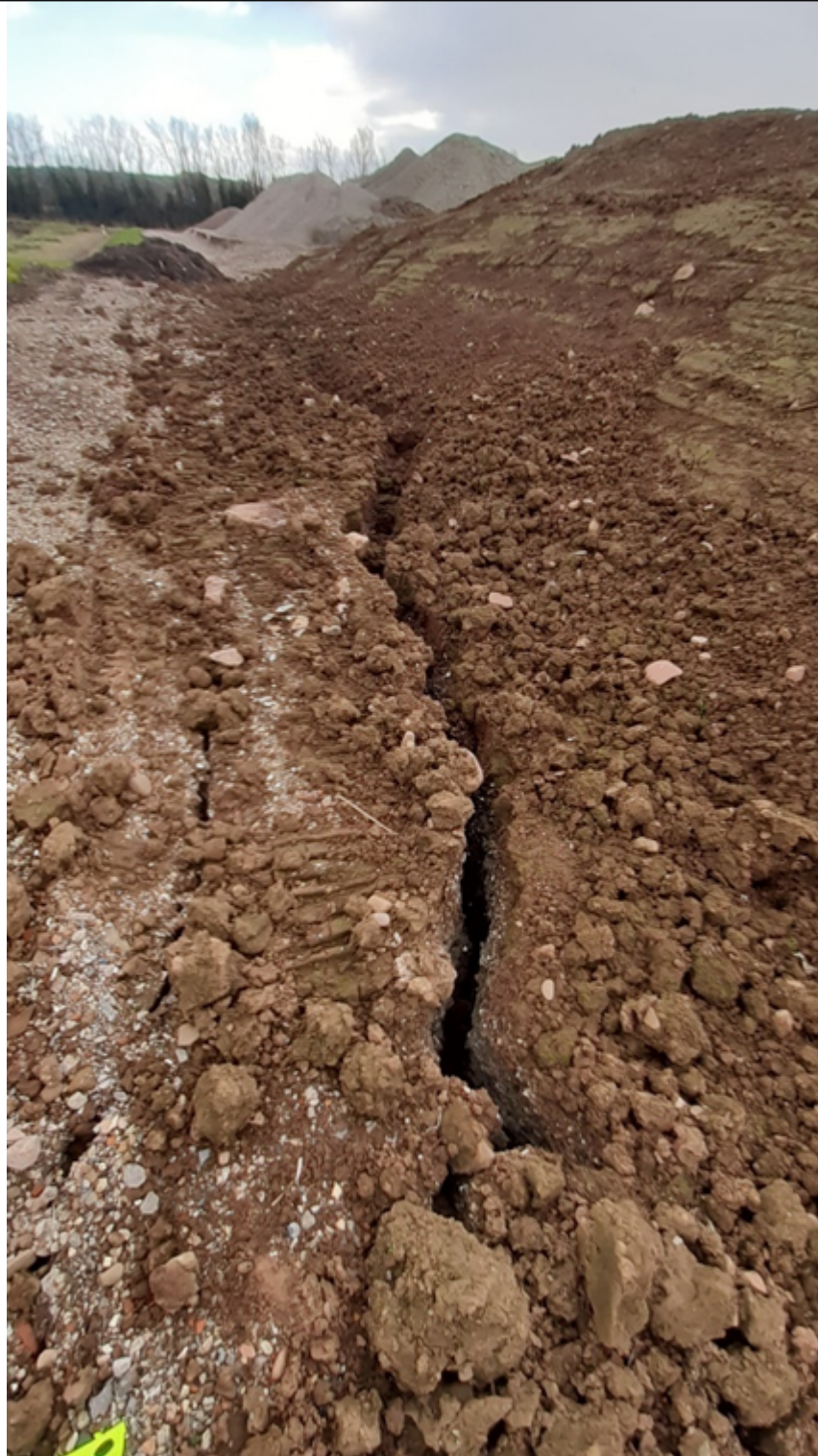
Picture 2 - Image of the soil pile with large cracks showing the slip zones on the 2nd of February 2022.
