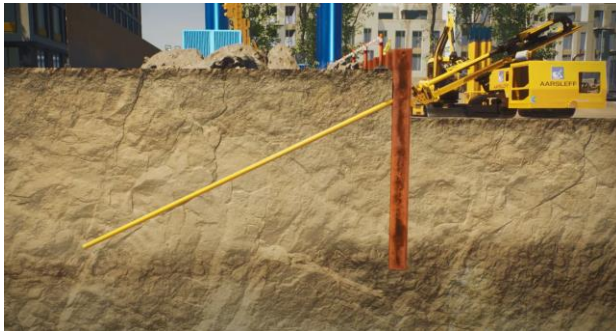
Fig.9 : Full bolt section in place
