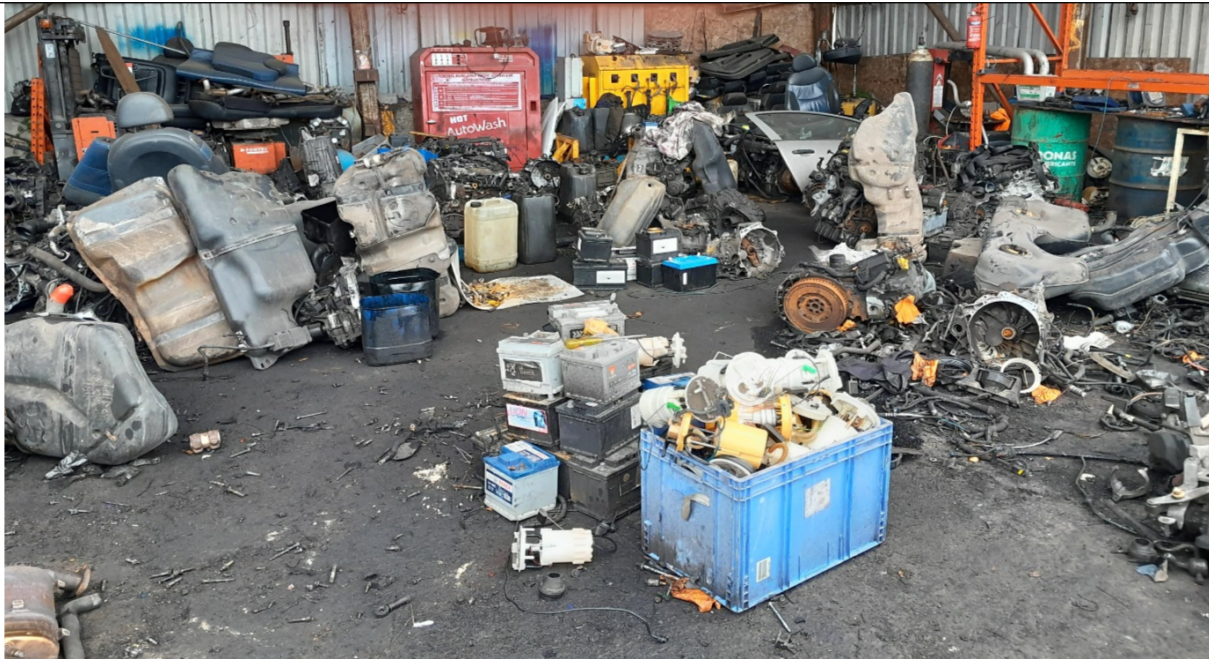
Photo 3 - Batteries witnessed stored outside of a sealed container
