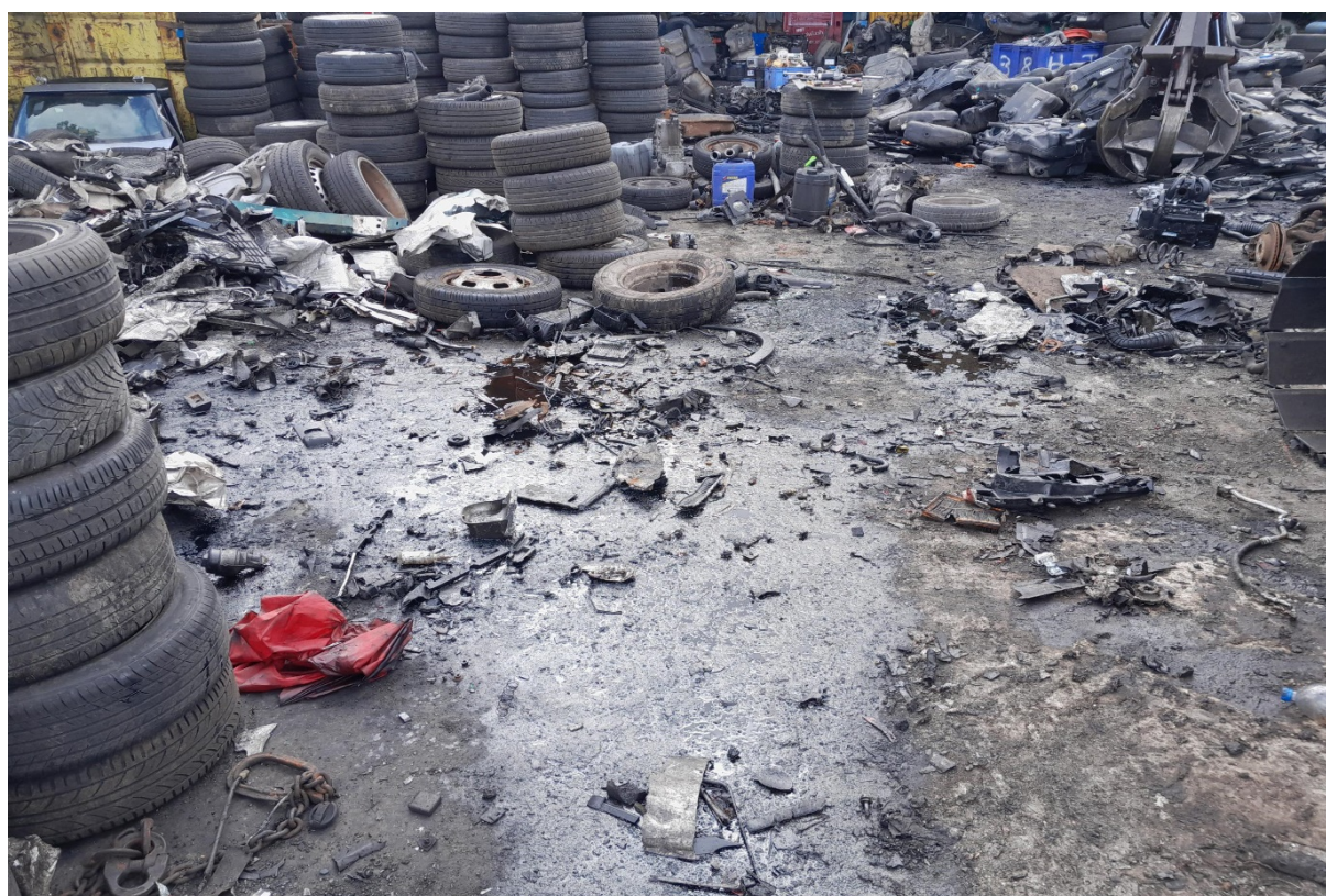
Photo 1 - Pooling of oil on flooring with no countermeasures in place
