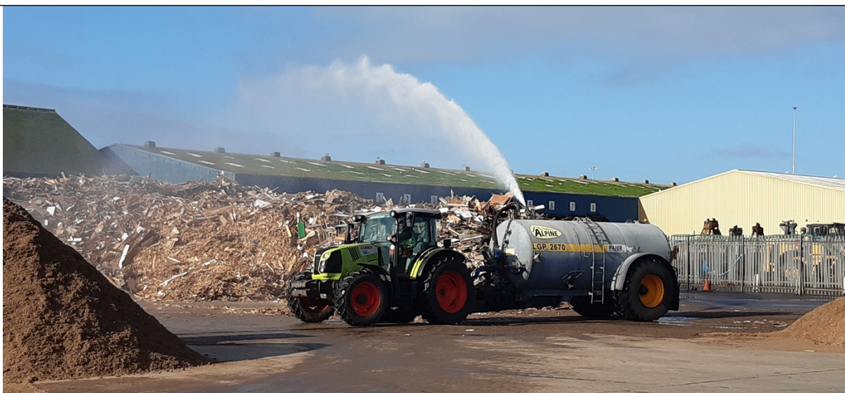
Photo 3 - On site water bowser for dust suppression and fire fighting purposes
