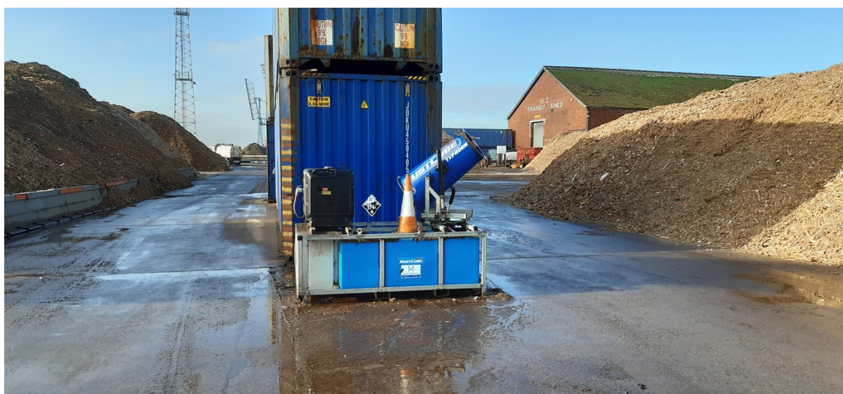
Photo 4 - Mist cannon to help minimise the presence of airborne dust
