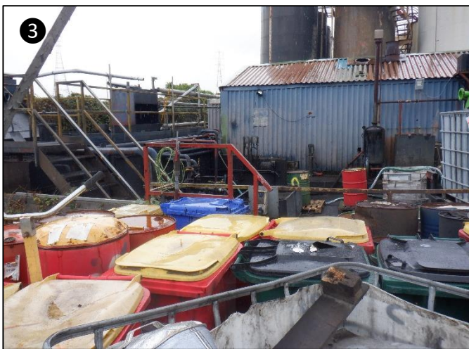
3 & 4: Bins/drums storing polluting liquid contaminated items not provided with secondary containment.
