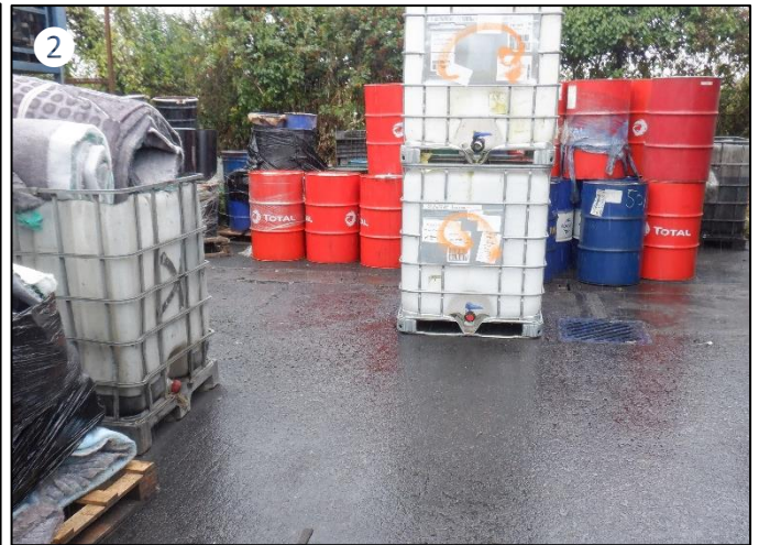
Photograph 1 & 2: IBCs storing waste oil/lubricant not provided with secondary containment.
