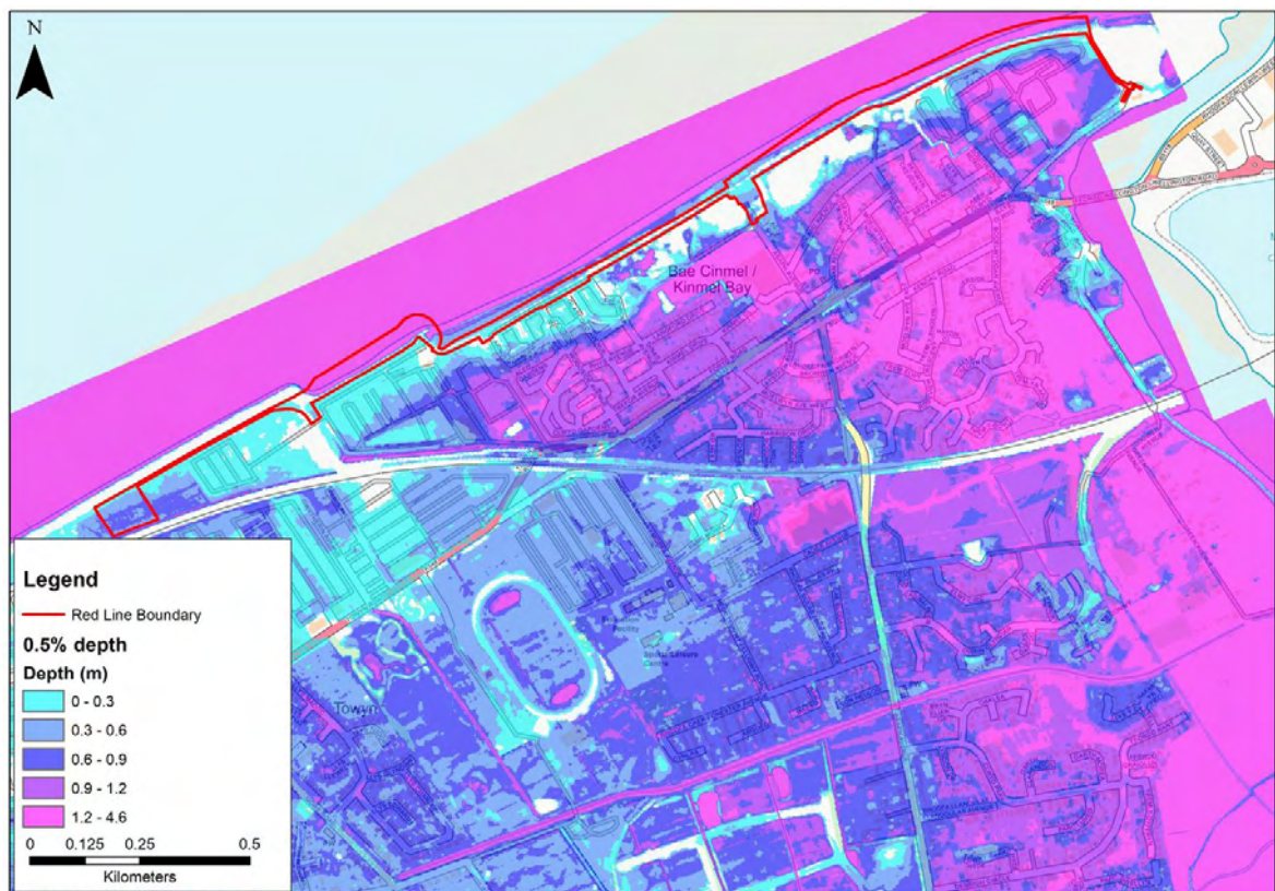
Figure 5-7 2121 0.5% AEP tidal flood event depth - post development
