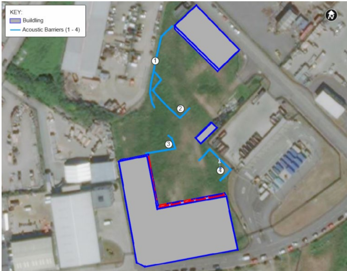
Figure 8: Embedded Mitigation - Acoustic Barriers
