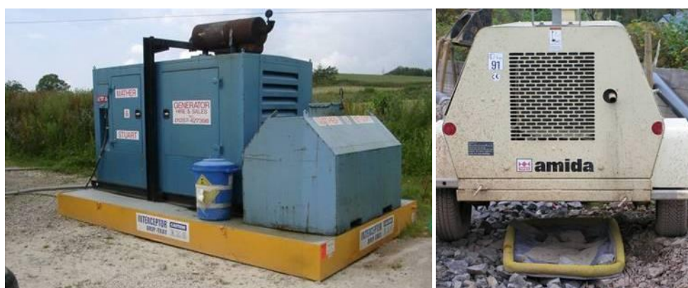
Figure 13: Generator on Drip Tray with Integral Separator / 'Plant Nappy' under compressor
