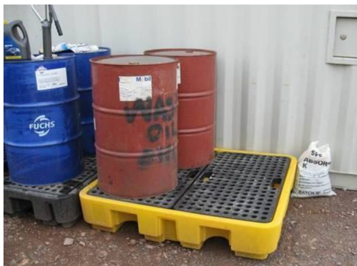
Figure 12: Barrels Stored on Drip Tray
