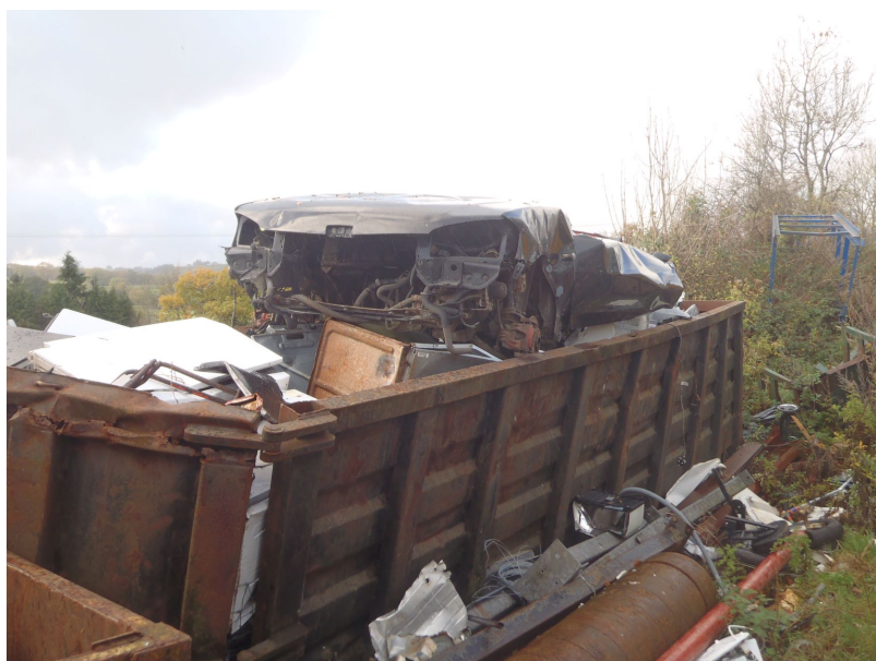
Undepolluted End-of-Life vehicle in skip on unmade ground
