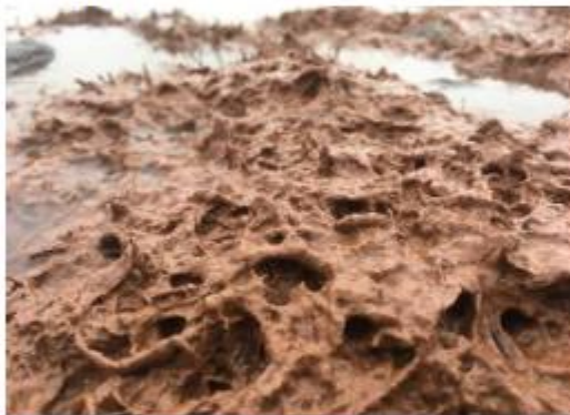
Close up FlocMat showing accretion of silt
