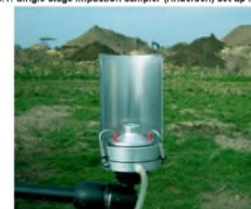
Photograph 5.1: Single stage impaction sampler (Andersen) set up in the field
