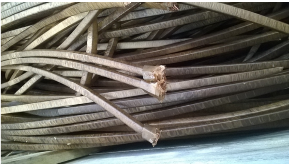
Photo 4: Copper windings in paper covering
