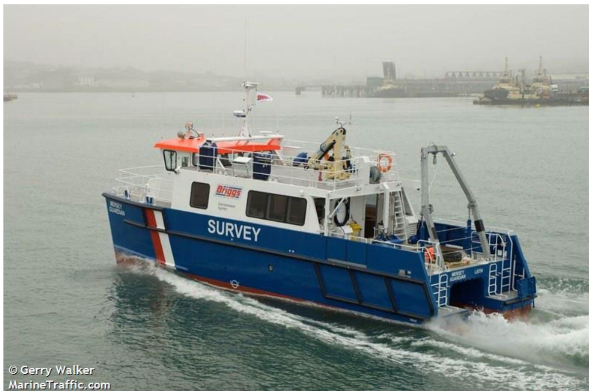
Figure 3. Image of the survey vessel, Mersey Guardian, which was used to carry out the acoustic survey of the Dee estuary on 27 May 2021. The Severn Guardian was used in the August survey and is almost identical. The major difference between the two vessels was the deployment of the sonar transducer: on the Mersey Guardian in May, the transducer was deployed on a pole mounted through the moon pool on the rear deck of the vessel; on the Severn Guardian in August, the pole was mounted on the port side in line with the foremost part of the aft deck.
