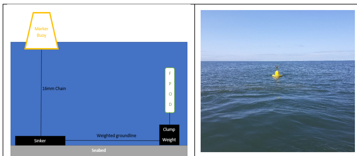
Figure 7. Schematisation (left) and deployment (right) of fixed acoustic mooring
